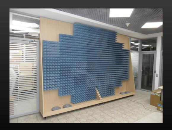
Radiation-absorbent material (RAM) to ensure magnetic field uniformity in the workspace
